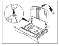
**3** Attach the extension cover on the back of the machine.
